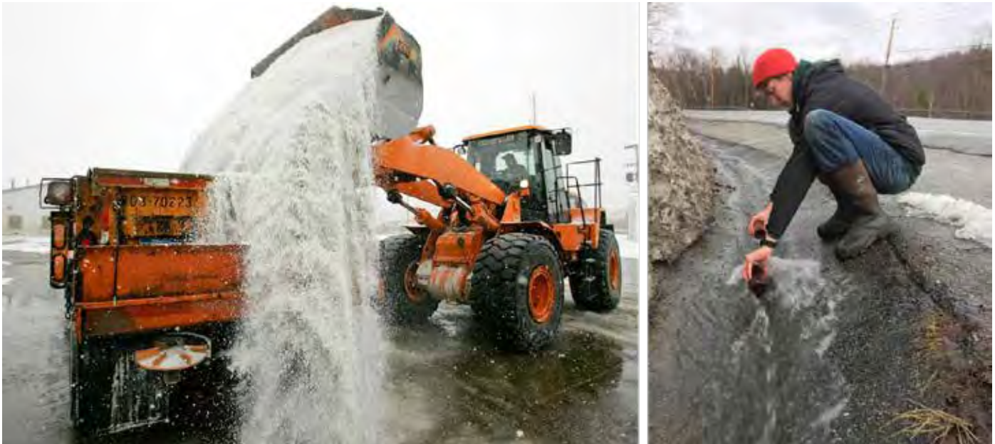
Rock salt (sodium chloride) being loaded into the back of a salt truck (left). AWI technician, Hunter Favreau, collecting a sample of direct road runoff from NYS Rt. 28/30 in the hamlet of Blue Mountain Lake in March of 2017. This sample contained over 700 mg/L of chloride, which is approximately 1,400 times the concentration of unimpacted surface runoff (right).
