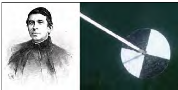
The Italian astronomer, Angelo Secchi (1818-1878), and the limnological tool named after him. Secchi initially developed the disk to measure the depths of Venetian Canals
